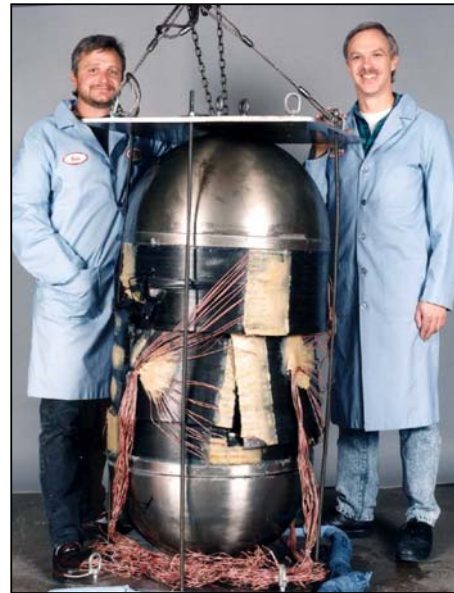
Figure 3.1 In the test, the cylinder failed at 37.9 MPa (5500 psi), within 3% of prediction.
