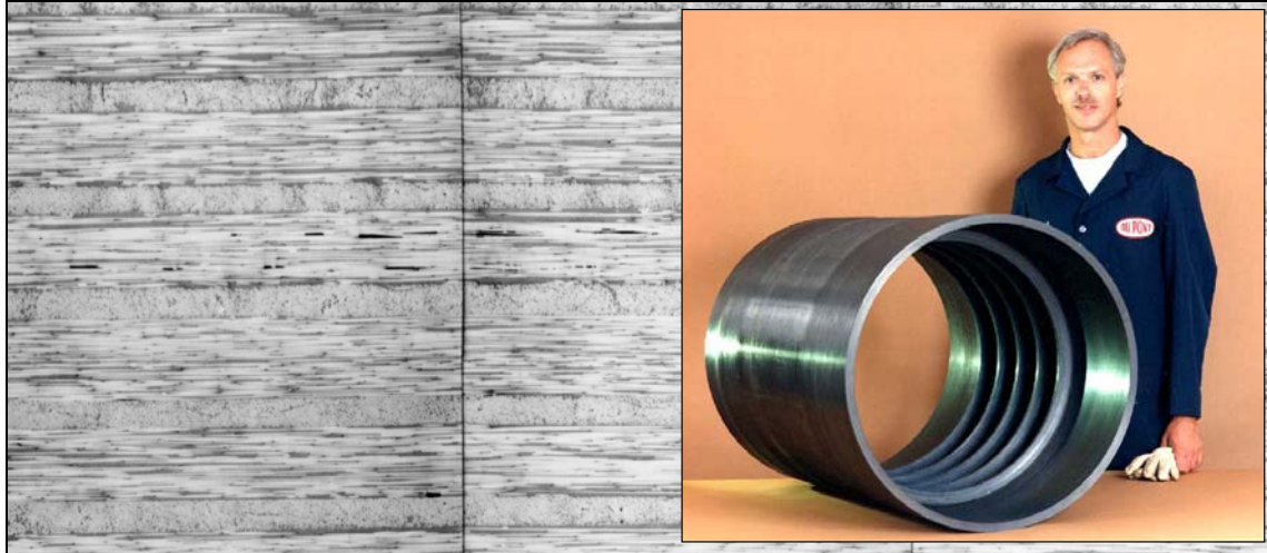
Figure 2.1 The APC-2/AS-4 ring-stiffened cylinder had a [90^{\circ}_{2.27/0}]_n laminate stacking sequence and five integral 90^{\circ} ring stiffeners. Quality was high with a 0.9% void volume fraction, no hoop waviness, and little axial waviness.
