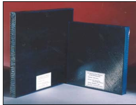
Figure 8.1 Primary bonding using thermoplastic in situ consolidation to place 76mm (3-in) tape on honeycomb core precoated with BRx-5 and FMx-5 adhesives.
