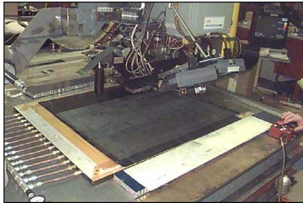
Figure 9.1 Cytec Engineered Materials 76mm (3-in) deposition head used to place Ti foils and IM-6/PEEK tape into a TiGr laminate with in situ consolidation
