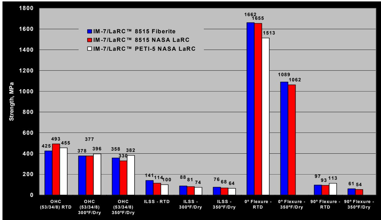
Figure 6 Strengths for IM-7/NASA LaRC™ 8515 compared with IM-7/PETI-5
