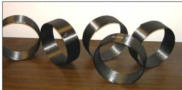
*Figure 10 The AS-4 carbon/NASA LaRC™ impregnated tow was filament wound into rings. This thermoplastic in situ consolidation process was completely out of the autoclave.*
