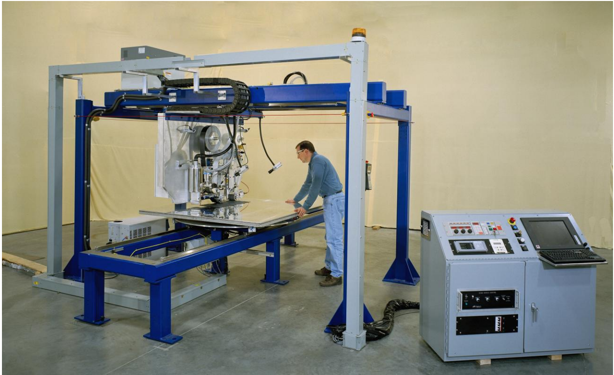
Figure 5: E-Beam Flat Tape Laying Head and Gantry
